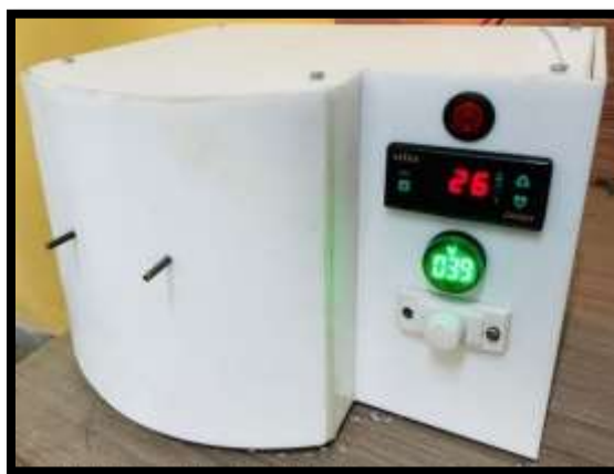
Figure 1. Actual Experimental Setup for microreactor based synthesis of cobalt ferrite
